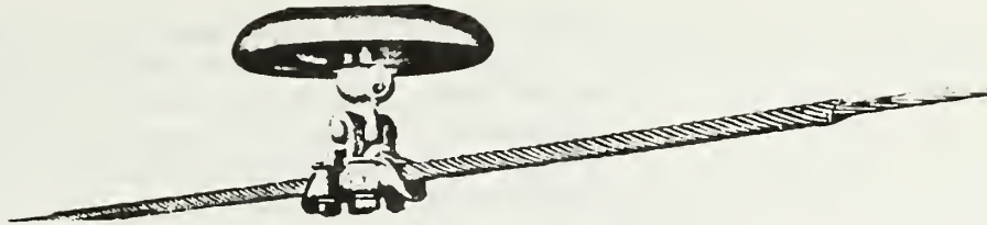
FIGURE XV-9: ARMOR RODS USED WITH SUSPENSION INSULATORS.
