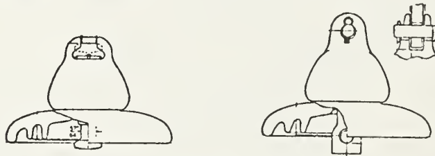
FIGURE XV-5: SUSPENSION INSULATORS - BALL AND SOCKET TYPE (LEFT) AND CLEVIS-EYE TYPE (RIGHT).
